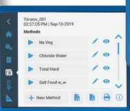
Customizable methods save electrode, titrant and sample titration settings so routine procedures can be repeated without additional setup or pre-work and methods can be shared among titrators using a USB flash drive.
