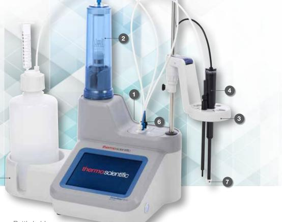
Paired with premium ROSS pH electrode, Orion redox and Orion ion selective electrode technology to provide a complete measurement system optimized for accurate, reproducible sample analysis.
